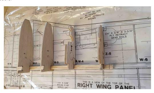
So this photo shows my mock up in construction. I've decided not to cover the top and bottom with 1/16 inch skin so the completed structure, still drying out, is below.
