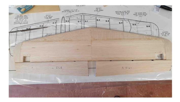
The instructions then call for the fin and rudder to be constructed but as they are on the 2<sup>nd</sup> sheet of drawings, I decided to build the wing next as I just had to turn over the sheet I was working on for the wing plan. Before starting the wing, I needed to get my head around how the various parts of the retracting main undercarriage would work. Take a look at the photo below.
